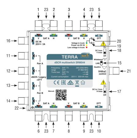
Figure 2. External view of the multiswitch SRM544
