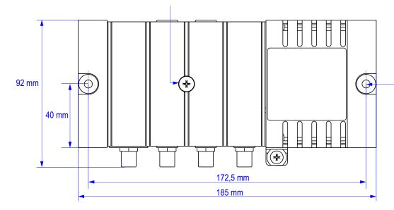
The amplifiers must be fixed with steel screws Ø 4-4.5 mm. The screws are not included in a package.
