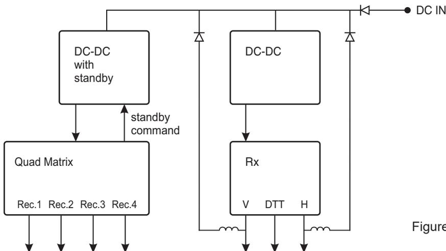
Figure 2. DC path diagram
