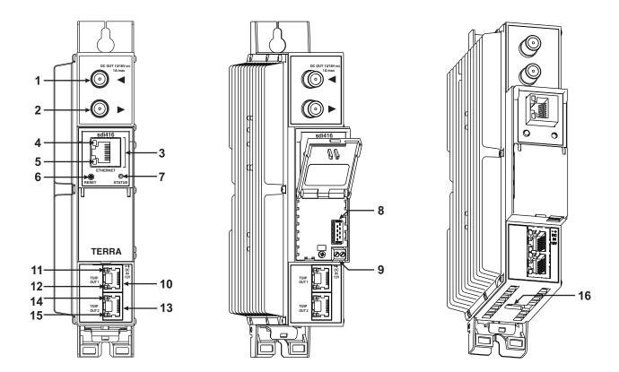
Figure 2. External view of the streamer
