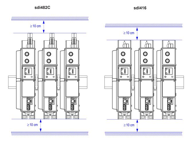
■ Mounting bracket on DIN rail should be connected to main potential equalization bus.
