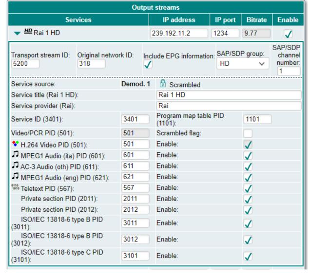
Figure 19. Extended settings of the output streams table
