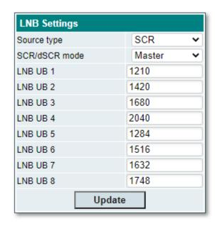
Figure 14. LNB settings table when "Source type" set to "SCR"
