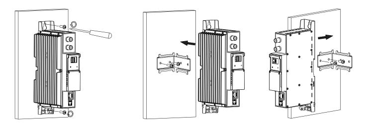
Figure 4. Mounting of the streamer
