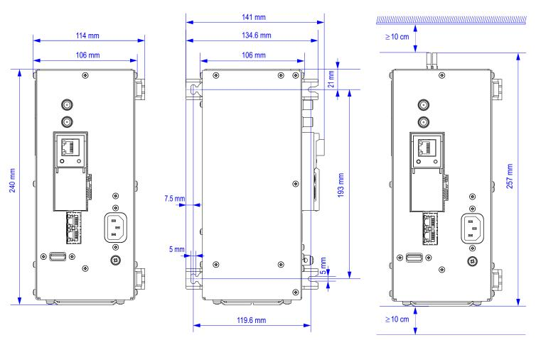
Figure 8. Mounting of the streamer
