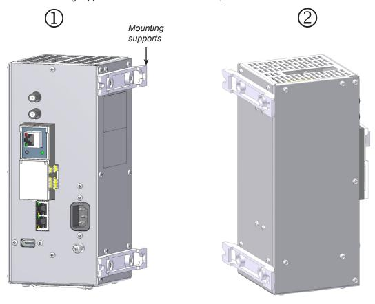
■ Free space of installed streamers must be at least 10 cm.
