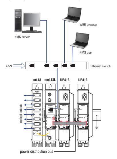
Figure 15. Application diagram of mo418L installation with redundant power supply and WEB/SNMP control possibility.
