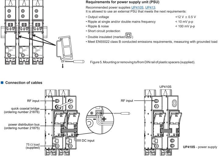
Figure 6 a. Powering of the transmitter via screw terminal block
